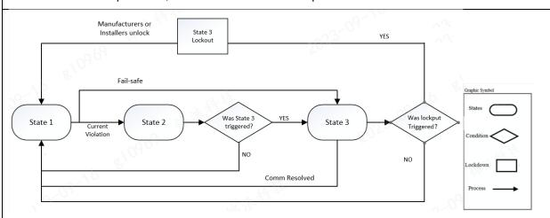
Ginlong G100 CLS was designed with a fail safe mechanism according to G100 Issue 2 2022, ensuring that in the event of communication failure or loss of source in any component, reducing the component generation to zero.
